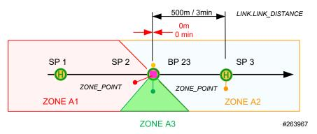
In this situation, border point BP23 is located on the path between SP2 and SP3 with POINT\_TO\_DISTANCE (SEL\_ZP\_LAENGE) = 0.
