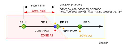
In this situation, border point BP23 is located on the path between SP1 and SP2 with POINT\_TO\_DISTANCE (SEL\_ZP\_LAENGE) = distance between SP1 and SP2.
