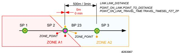
In this situation, border point BP23 is located on the path between SP2 and SP3 with POINT\_TO\_DISTANCE (SEL\_ZP\_LAENGE) = 0.
