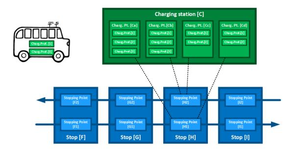
The charging points have a joint supply line (medium voltage), which is transferred to the charging voltage for the charging points. In this case, the charging station corresponds to a stop and the charging points are allocated to its stopping point.
